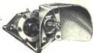
Rear power take-off drive.
