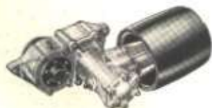
Rear power take-off pulley.
