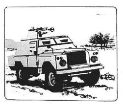
Based on the 109 in. military Land-Rover chassis, the Shorland armoured car provides an effective degree of protection against small arms fire and improvised ambush weapons. With a 360° rotation gun turret, having mountings for a .300 in. Browning or 7.62 mm. general purpose machine gun, and observation and escape hatches, the vehicle takes a crew of three, and is suitable for operation in all climates.
