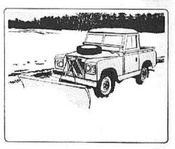
A 'V' type snowplough for use at speeds of up to 25 m.p.h. Easily fitted or removed from the Land-Rover with no structural alterations. Raised and lowered mechanically.
