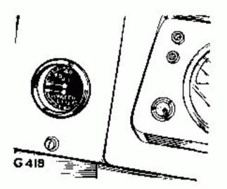
Water thermometer and oil pressure gauge
