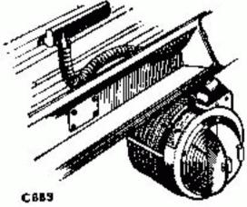
In warm weather, the heater can c<sup>s</sup> be used for air circulation with the water supply cut off by means of the tap on the inlet pipe under the bonnet.
